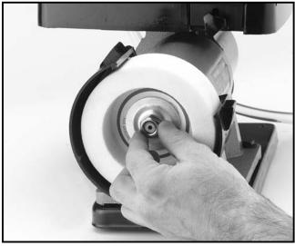
Figure 10. Removing dry wheel.
